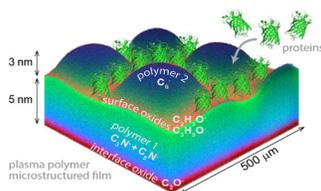
Plasma polymer films are promising biointerface materials with applications for future tissue engineering, biosensing and more. To optimize film functionality, such as protein binding, it's necessary to understand how the competing mechanisms during the deposition of reactive species on the surface of materials affect their chemical characteristics.
